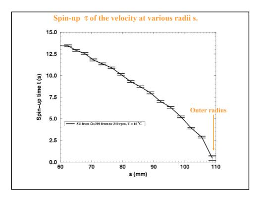
•Azimuthal velocity  $u_{\phi}$  as a function of *t*, *s*, after a spin-up: (Greenspan, 1968)  $u_{\phi}(s,t) = s \Delta \Omega \exp(-\frac{t}{\tau})$  $-\frac{(1-s^2/R^2)^{3/4}}{E^{1/2}\Omega}$  $\tau \ \alpha \ E^{-1/2} \quad \text{for} \frac{\Delta \Omega}{\Omega} < 1 \text{ (linear theory)}$
